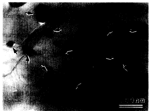
Fig. 4. Transmission electron micrographs for Al_2O_3/5 vol% Cu nanocomposite, hot-pressed at 1450°C for 1h.
